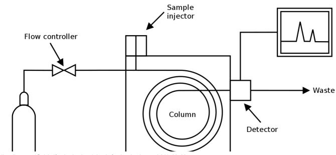
So, when gas, as a mobile phase, is passed through the coiled tubes, different flavor molecules have different affinity towards the stationary phase.
